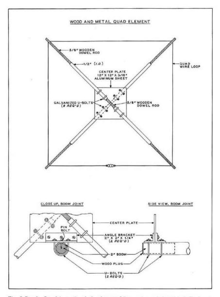
Fig. 3 Sturdy Quad is made of aluminum tubing and wood dowel rod. Each arm of array is made of sections of tubing and rod. Arms are then attached to a 12'' x 12'' aluminum center plate with U-bolts. One arm is placed on each side of the plate. The assembly is held to the 2'' aluminum boom by means of double angle brackets and U-bolts. Assembly is pinned to the boom by bolts running through the bracket, boom and wood plug.
