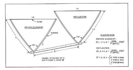
Fig. 3 Delta Quad is formed of triangular elements inverted and supported at the apex. The wings may be made of aluminum tubing and are about 1/3 wavelength long. The top portion of the loop, or triangle, is made of wire. Base angle of the delta element is 75 degrees and both wings may be grounded to the metal boom. Off-center, gamma match feed is suggested, using the gamma dimensions and spacings given in Fig. 7, Chapter VI as a starting point.
