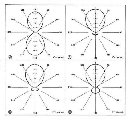
Fig. 7 Polar plots of 3-element Quad show good F/B ratio at design frequency.
