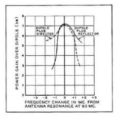
Fig. 12 As operating frequency of parasitic array is varied the power gain over dipole drops rapidly as the parasitic element becomes resonant. The shape of the gain curve thus depends whether parasitic is a reflector or a director.
