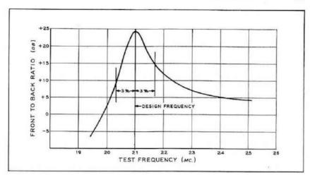
Fig. 14 Front-to-back ratio drops rapidly as the Quad antenna is operated off-frequency. Even so, Quad qualifies as "broad band" antenna, as it retains good F/B ratio over span of approximately 6% of design frequency.
