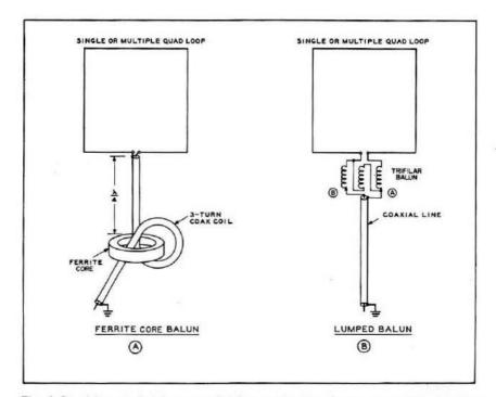
Fig. 4 Quad loop is fed from coaxial line and balun. Ferrite core (A) is Indiana General CF-123 (Q-1 material), 2.4" outside diameter. Information may be obtained from Indiana General Corp., Crow Mills Rd., Keasby, NJ 08832. Trifilar air core, coil balun (B) is shown in Figure 5.
