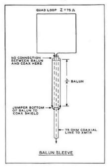
Fig. 6 Unbalanced coaxial line may be attached directly to Quad loop with aid of balun sleeve placed at top end of line. Sleeve and outer conductor of line form a quarter-wavelength transformer having a high impedance across the open end (top). Both terminals of the coaxial line are isolated from ground.
