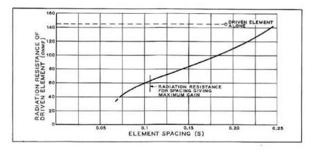
Fig. 7 The radiation resistance of a two element Quad varies between 40 ohms and 140 ohms as element spacing increases from 0.07 wavelength to 0.25 wavelength. Radiation resistance of Quad may be adjusted to 52 ohms by making spacing 0.08 wavelength, or 72 ohms with 0.13 wavelength spacing.
