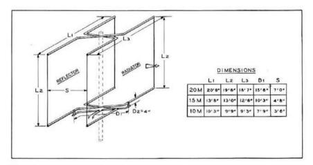
Fig. 4 The Swiss Quad is an all-driven array having a unidirectional field pattern similar to the regular Quad. The elements may be grounded to the supporting mast at the top and bottom. A T-match feed system is used. The Swiss Quad may be fed with an open wire (TV-ribbon) line and antenna tuner or a balun and coaxial line. T-match is adjusted for lowest SWR.
