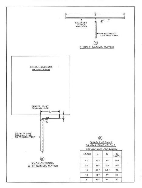
Fig. 7 Popular gamma match may easily be employed with Quad antenna. Gamma is used to match unbalanced coaxial line to balanced antenna system (A). Same configuration is used with Quad, except gamma is made of wire, and spacing between gamma wire and Quad loop is quite small. Gamma dimensions for all bands are given in chart C. Gamma capacitor setting will be approximately 90% of value shown. For power up to one kilowatt, small wide-spaced receiving type capacitors may be employed.
