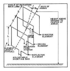
Fig. 1 Three element Quad makes use of open director stub to provide capacitive reactance (see Fig. 9E). However, director may be self-resonant, or undersized with closed stub. See Fig. 6 for typical dimensional data.
