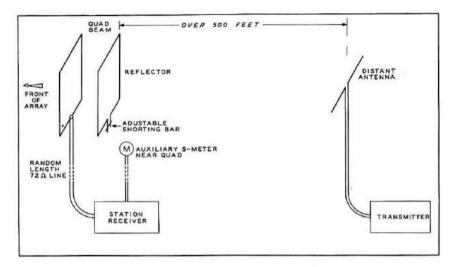
Fig. 1 Quad antenna may be adjusted for maximum front-to-back ratio with this test set-up, making use of your receiver and the transmitter of nearby ham. The distant test antenna should be horizontal for optimum results.
