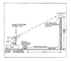
Fig. 4 Antenna measurements can be made with accuracy at 144 mc. Test antenna is aimed upwards at a distant field strength meter to reduce the effects of ground reflection. Pattern and gain figures are plotted.
