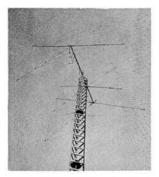
Experimental three band concentric Quad uses close-spaced reflector for 28 and 21 mc and wide-spaced reflector for 14 mc. Average impedance of all three beams is close to 75 ohms and low impedance coaxial transmission line is used as feed system for antennas.
