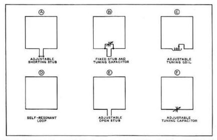
Fig. 9 Parasitic element of Quad may be resonated by shorting stub (A) and (B), or by adjustable coil (C). Optimum adjustment is achieved by making the parasitic element self-resonant (D). Adjustable open stub (E) or series tuning capacitor (F) are sometimes used for stub adjustment.
