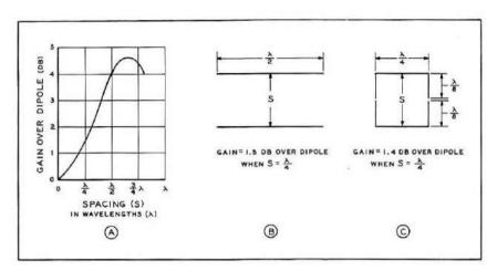
Fig. 5 The power gain of two half-wave elements operating in a vertical stack is shown in graph A. At a separation of one-quarter wavelength, the power gain is 1.5 decibel. A fraction of this gain is lost when the ends of the elements are folded towards each other as shown at C. Since there is no current flowing at the element tips, they may be connected together to form a closed loop. The loop may be square or diamond shaped and is broken at the bottom for feeding.
