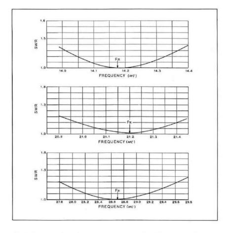
Fig. 4 Properly adjusted Quad antenna shows 1.0/1 SWR at resonant frequency of driven element, with SWR curve rising smoothly and gradually each side of resonance point. Bandwidth of Quad is ample for complete coverage of 14, 21, or 28 mc band. Three band Quad exhibits similar curves. Use of gamma match with Quad antenna permits quick and easy adjustments.
