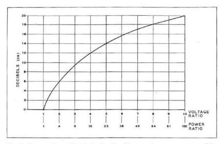
Fig. 1 Power gain and front-to-back ratio of beam antennas are expressed in terms of decibels. Relationship between decibel and voltage or power ratio is shown in this chart. Most receiver S-meters have scale that is calibrated in decibels but which bears no relation to true measurement.
