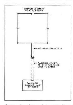
Fig. 2 Low impedance points of the X-Q array are located at the corners of the loop making feeding problem more difficult than in the case of the simple Quad. A simple and effective solution is to feed X-Q loop at the center of the lower section (high impedance point) with a quarter-wave matching transformer. This permits a balanced, low impedance transmission line to be coupled to the antenna. Balun or tuning unit is used at transmitter (unbalanced) for pi-network output circuits.
