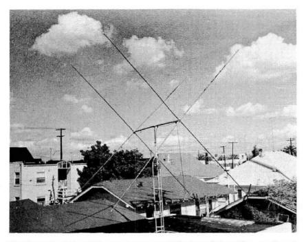
The 14 mc single band Quad antenna mounted atop a flat roof for experiments.
