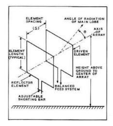
The spacing between the two loop elements is adjustable, and the supporting framework is made of wood to eliminate spurious resonance effects in the structure. The parasitic element is broken in the same manner as the driven element permitting adjustment by means of a variable shorting bar. Field strength readings are taken at an extreme distance from the array and the height above ground of the field strength meter is adjustable.
