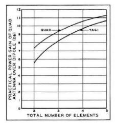
Fig. 9 A comparison between the Yagi and the Quad antenna. For an equivalent number of elements, the Quad exhibits a power advantage over the Yagi of about 1.7 decibel. Expressed in terms of boom length, the Quad may have about twothirds the boom length of a Yagi for equal power gain.
