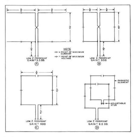
Fig. 1 Expanded Quad (X-Q) antenna is derived from Lazy-H array (A). Ends of "H" are folded back (B) and cross-over feed system is eliminated (C). The X-Q loop provides a power gain of about 5 decibels over a reference dipole. Two element X-Q array provides power gain of 9.5 decibels over a dipole.
