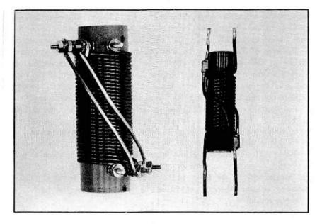
Fig. 5 Air core balun at left is good for 1000 watts PEP power level. Jumpers connect windings in proper sequence. Coil termination (A) is at lower right with termination (B) at lower left. Ferrite core balun is at right.
