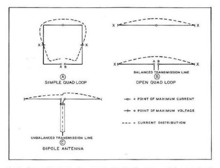
Fig. 1 Current distribution is symmetrical in Quad antenna as it forms a closed system (A). Unequal and improperly phased currents may flow in a dipole antenna (C) as no electrical connection exists between dipole halves.
