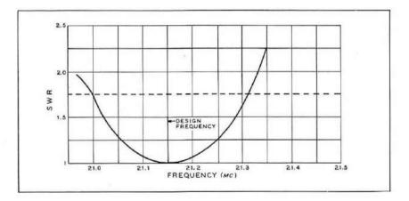
Fig. 4 Three element Quad array exhibits a narrow bandwidth when elements are tuned for maximum gain and optimum front-to-back ratio. Experimental 21 mc. Quad showed 300 kilocycle bandwidth over which SWR on transmission line remained below 1.75/1. SWR increases rapidly on high frequency side of resonant frequency as the parasitic director nears a resonant condition.
