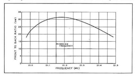
Fig. 5 F/B ratio of three-element 21 mc. Quad is better than 25 db. across band.
