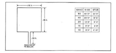
Fig. 6 Mini-Quad loop, suitable for use on the low frequency bands, is made of smaller-than-usual Quad, with excess wire folded into a balanced transmission line. Total wire length is equal to that of a full size Quad element. Bandwidth of Mini-Quad is sufficient for 40 meter band and for 200 kc portion of the 80 meter band. Stub may be adjusted to change resonant frequency.
