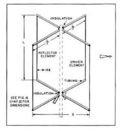
Fig. 5 The G4ZU Birdcage Quad uses two Quad loops folded back at the center so that the top sections act as supports for the vertical wires. Reflector and driven element loops are individually insulated from the supporting mast. The reflector loop uses a stub, or may be made oversize. Driven element is fed from a balun and coaxial transmission line.
