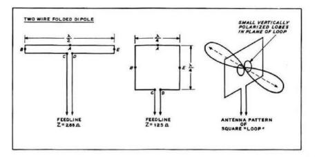
Fig. 4 The folded dipole may be formed into a square loop having two parallel elements, one above the other. The pattern of this loop is horizontally polarized with two small vertically polarized "ears" at right angles to the main lobes. This loop produces a power gain of about 1.4 decibel over the field of the dipole antenna (3.5 decibel gain over isotropic). Loop impedance is about 125 ohms.
