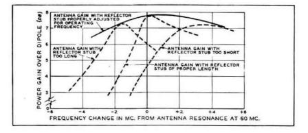
Fig. 13 When Quad employs parasitic reflector greatest operational bandwidth occurs on high frequency side of resonant point. Quad may operate efficiently plus or minus 3% of design frequency as shown above if the reflector element is retuned for off-frequency operation of the array.
