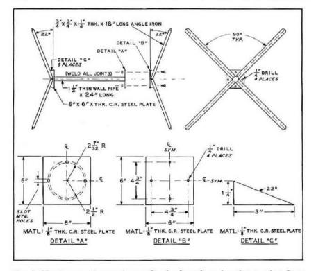
Fig. 4 Metal support for two element Quad reduces boom length to two feet. Structure is made in two parts so that Quad elements may be assembled on the ground and carried to top of tower for final assembly. Made of welded pipe, the Quad "spider" should be given two coats of paint before use.
