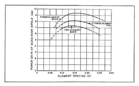
Fig. 2 Three element Quad shows power gain of about 9.3 decibels at element spacing of 0.15 wavelength. Gain is fairly constant for spacings of 0.13 to 0.22 wavelength and averages about 2 decibels better than 2 element Quad.
