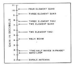
Fig. 3 Gain "ladder" shows the relative power gain in decibels of popular antennas. Two element Quad provides almost as much gain as three element Yagi. The four element Quad is "king of the band". Gain is compared against dipole antenna (0.decibel).
