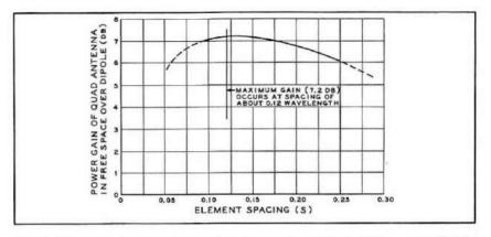
Fig. 6 The gain of a two element Quad array is constant within one decibel for element spacings of 0.08 wavelength to 0.22 wavelength. Maximum gain figure of about 7.4 decibels occurs near the 0.12 wavelength spacing. As the Q of the Quad element is low, the spacing is not a critical factor in the design of the array.
