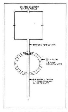
Fig. 4 Q-section, half-wave balun and coaxial line provide unbalanced feed system for pi-network transmitters. Balun provides 208 ohm termination point for 72 ohm line, and adjustable Q-section steps impedance up to several thousand ohms, suitable for high impedance feed point of X-Q.
